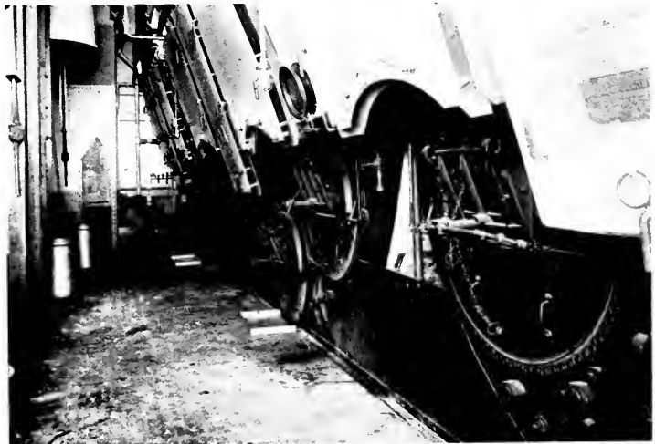
Fire-room of the steamer "Lieutenant Demissiessy," showing arrangement of Coen furnace fronts and burners.
